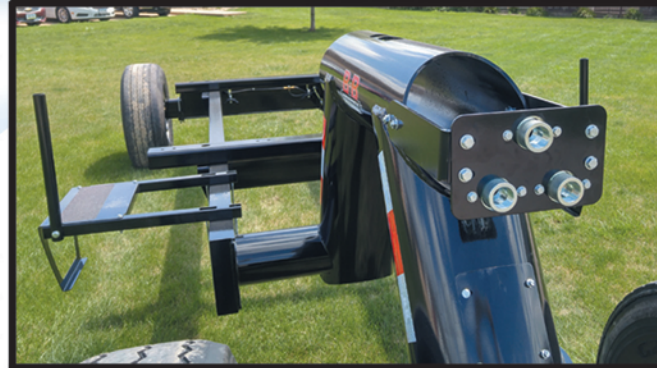
Round pipe neck for added strength & easy hose feed.
