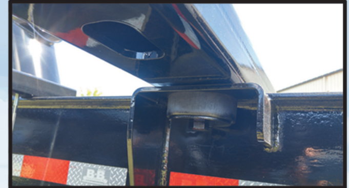
Bolt-on crossmembers repositionable with 1 1/2" thick rubber washer to help absorb shock and allow crossmember to flex.
