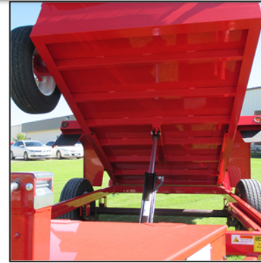
Cylinder lift on 5,000 GVW.
