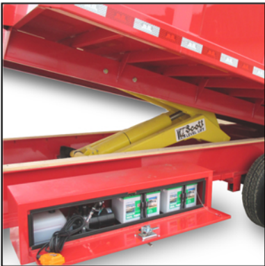
Battery & power unit storage.
