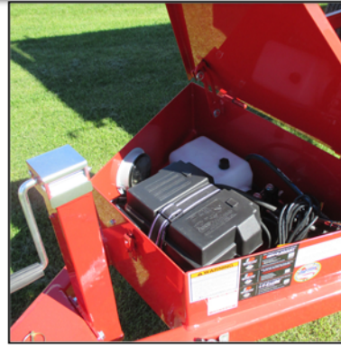
Battery and pump storage.
